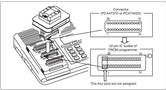
Figure 3.2 Attaching the adapter to a PROM programmer (PCA4738D or PCA7402D)
